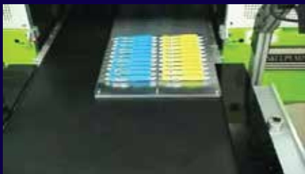
Accepts part caddies - Holds your parts as it rides into the machine
